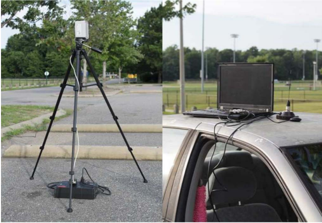
Fig. 5. Experimental setups of (left) a roadside AP and (right) a vehicular rogue AP.
